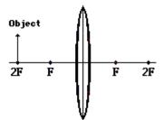
Ray diagram for he image of an object between 2F and F is:
